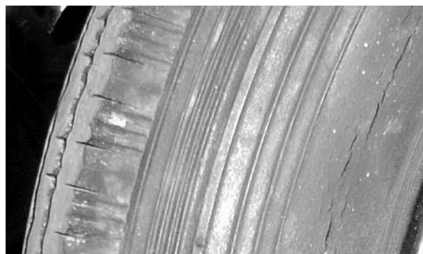
Example of a tyre with plenty of tread but whose cracked sidewall shows that it is too old to use.
