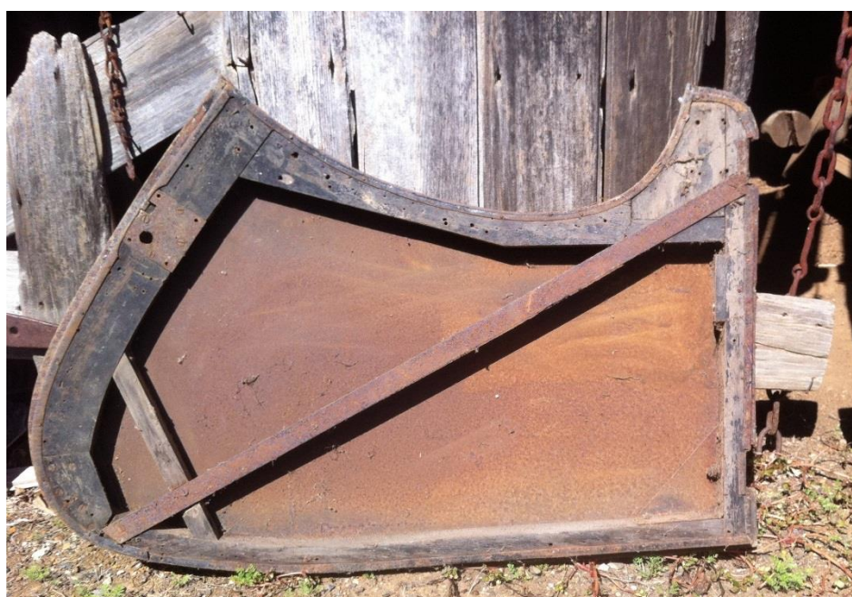
Later solid timber in door complete with strapping.
