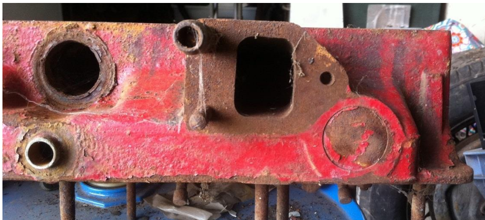
Cylinder head showing welch plug in the converted 90HP : P/N 566 -small valves to 100HP large valves.
