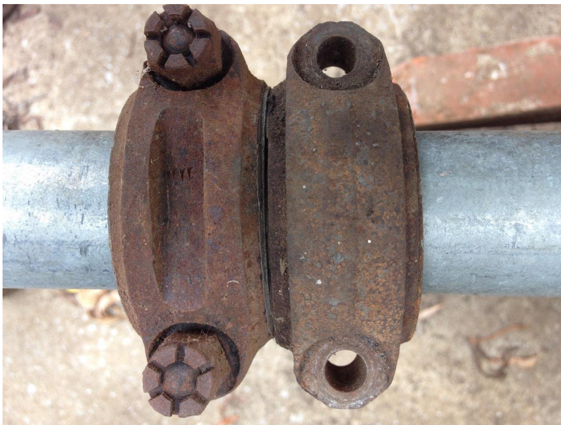
Big end caps early engine vs. later engines the early caps were the design of Frank Ashby weight saving same strength but more machining so dropped as a cost cutting move by Abington works as was the laminated timbers The diff housing was also changed some time 1949 around chassis no. 4118. #
