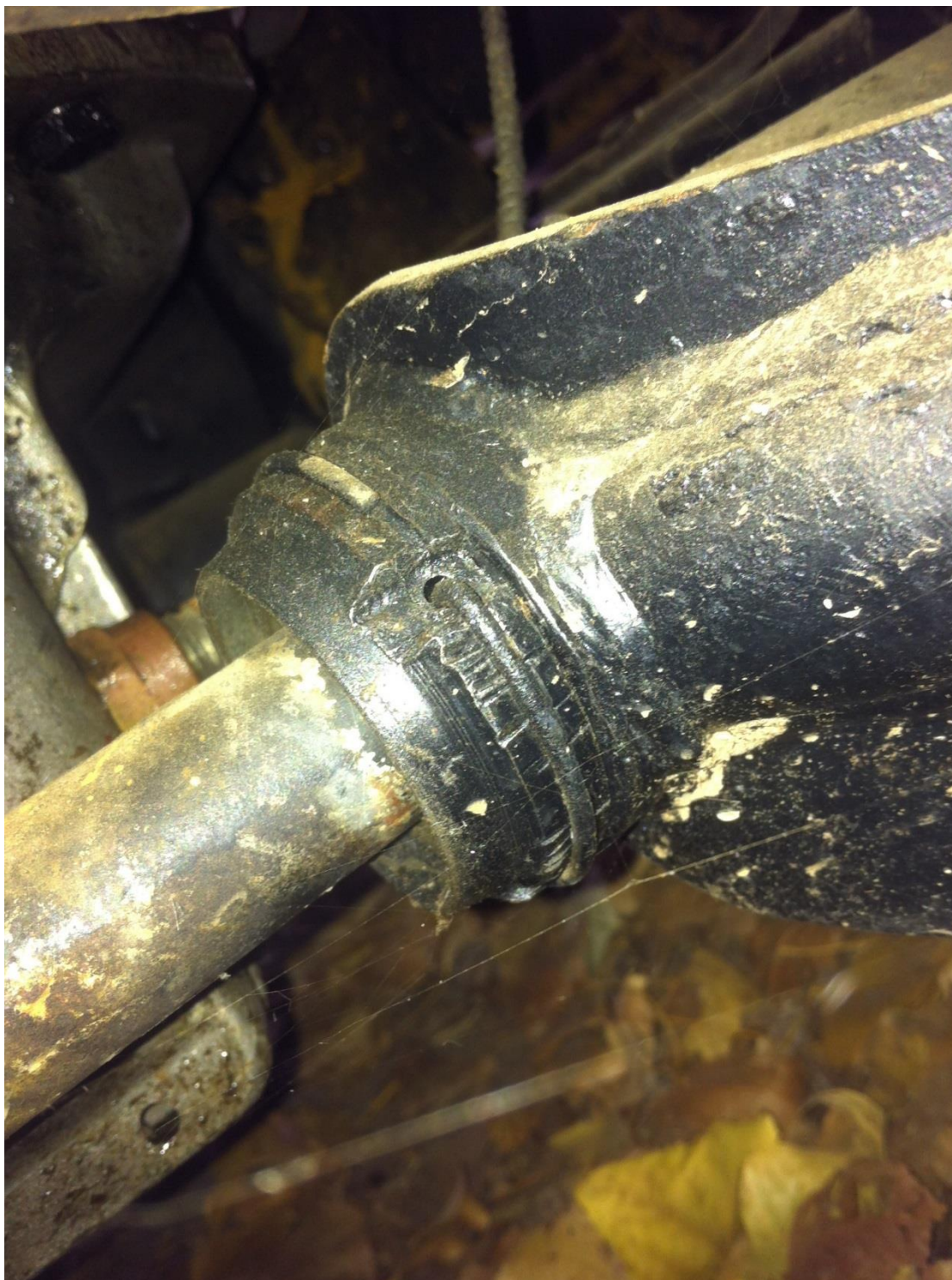
Ring nut lower rear strut, note extra width.
